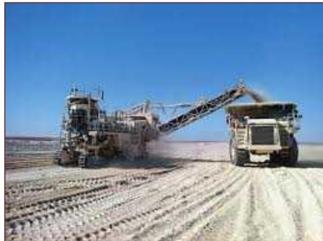
Photo: Surface miner loading haul truck
